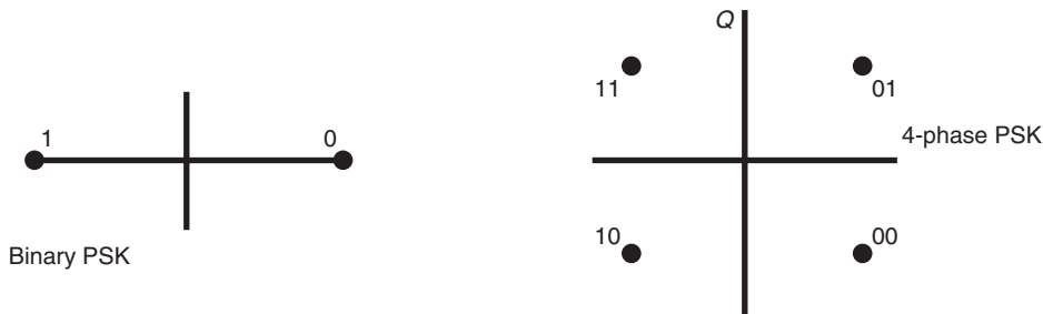
Figure 3.15 Phasor constellations for BPSK and QPSK.
